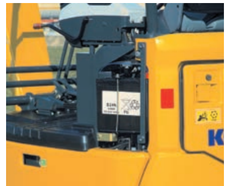
Left bonnet: easy access to the battery
