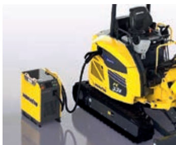
Komatsu off-board fast charger (Input: 400 V / 63 A) is standard
